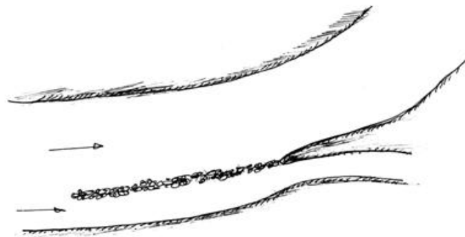
Figure 5. Typical layout for traditional canal intakes
